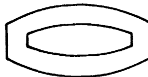
Fig. 28.3 Compaction of granular material around an already preformed core.
